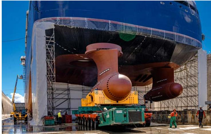
**THE** final stages in the construction of Ponant's *Le Commandant-Charcot* have begun, with the ship arriving in Saint-Nazaire to be fitted with Azipod propulsion systems.
